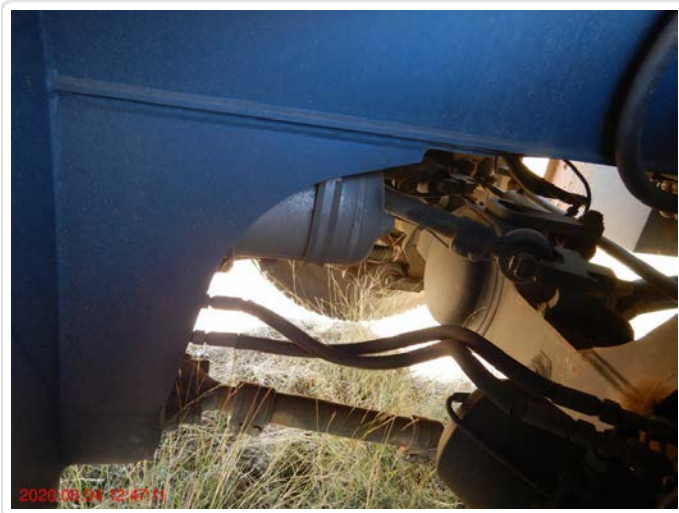
Brake Valves Various braking valves no issues evident
