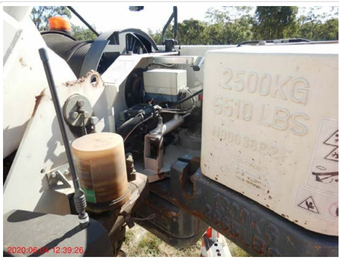
Leaks No leaks evident around the winch area
