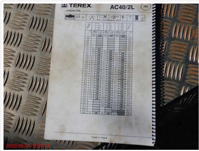
Load Chart Reference Number Full set of load charts available. applicable chart for function testing attached. other duties visually confirmed to the RCI (Computer)
