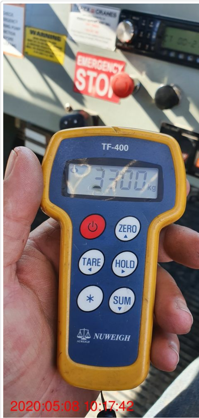
Line Pull Test - Load RCI
