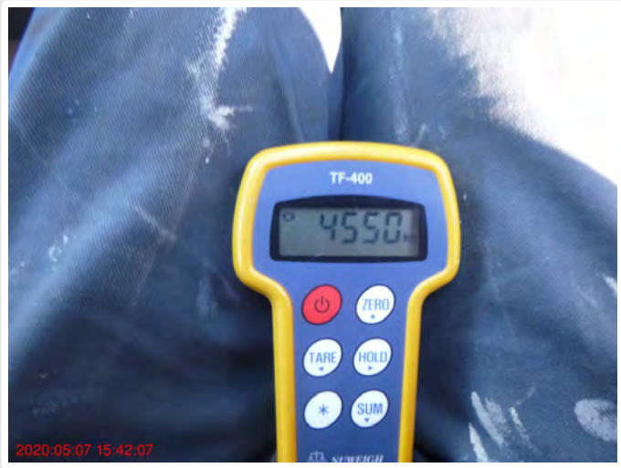
Line Pull Test - Load Measured
