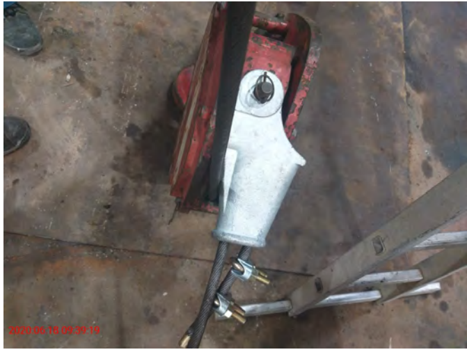
Correct Assembly and Connection of Hoist Rope Socket
