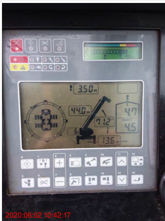
Line Pull Test - Load RCI
