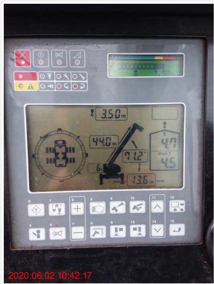
Line Pull Test - Load Measured
