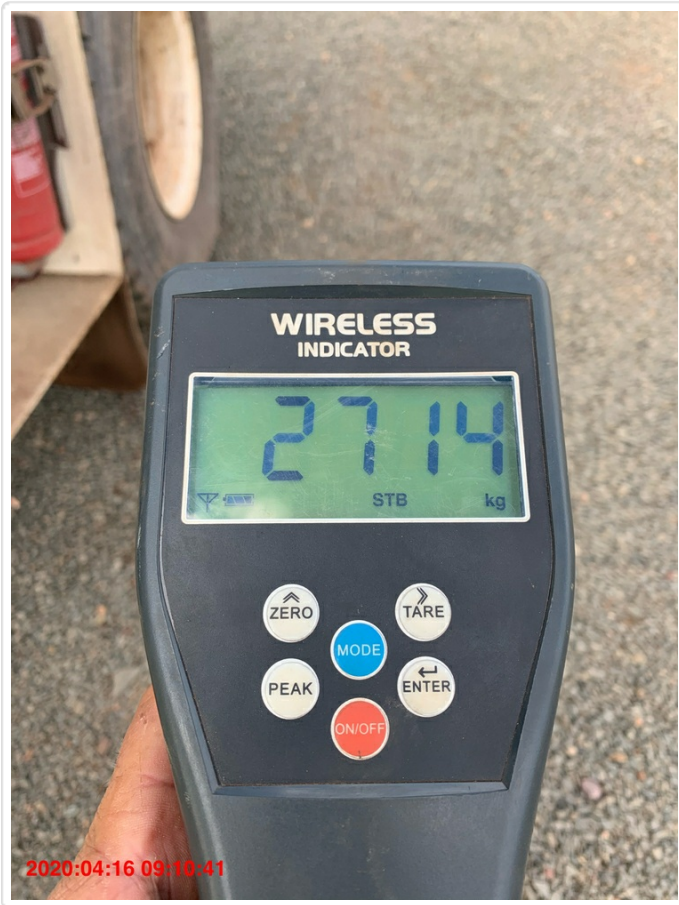
Rated Load - Boom Fully Extended - Load Measured LOAD EXCESS OF RCI
