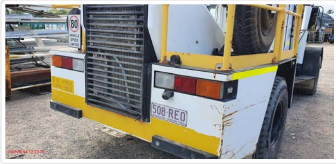
Counterweight Hazard Striping Faded hazard stripes
