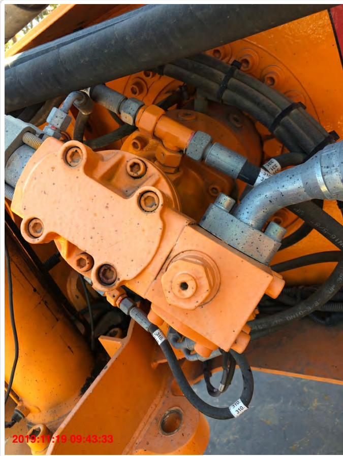
Main Winch Motor
