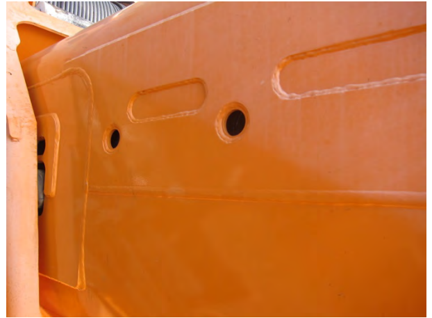
Photo 4: Boom stiffener and butt area
