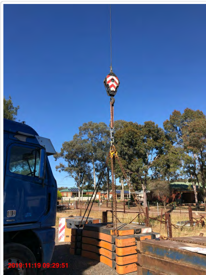
Line Pull Test - Load Measured
