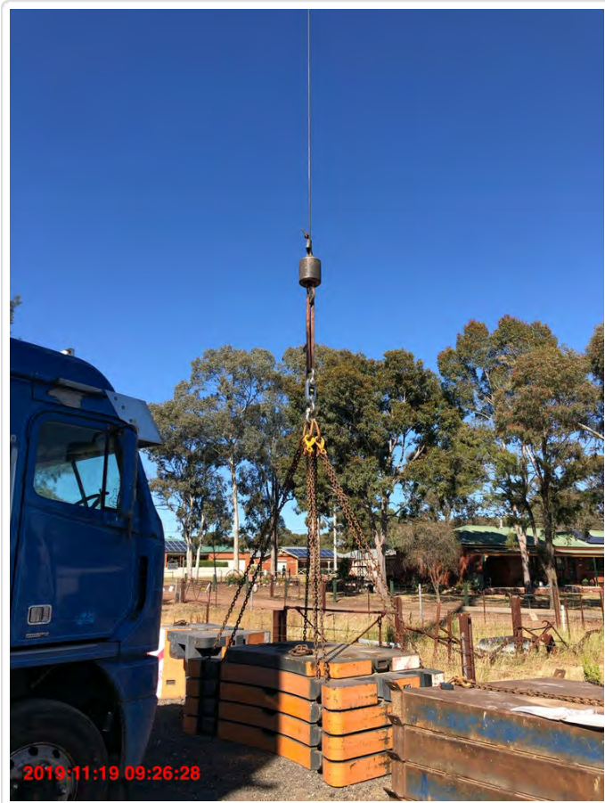
Line Pull Test - Load Measured
